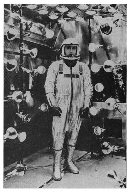
**COOL MAN** in a heat chamber, Scott tests five-layered aluminized space suit he worked on, says, "A man could go to the moon and back in it."
