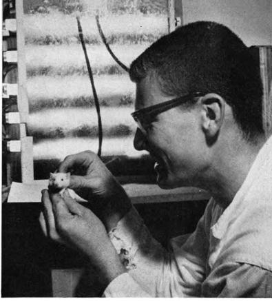
"A TOTAL BIOLOGICAL WORLD" is what Brian Tiep, eighteen, calls his photo-synthetic gas exchanger. Algae in tank behind him convert carbon dioxide to oxygen, which is piped to airtight cage containing a rat. Rat produces carbon dioxide, which feeds algae. Space travelers may use such systems to provide oxygen.
