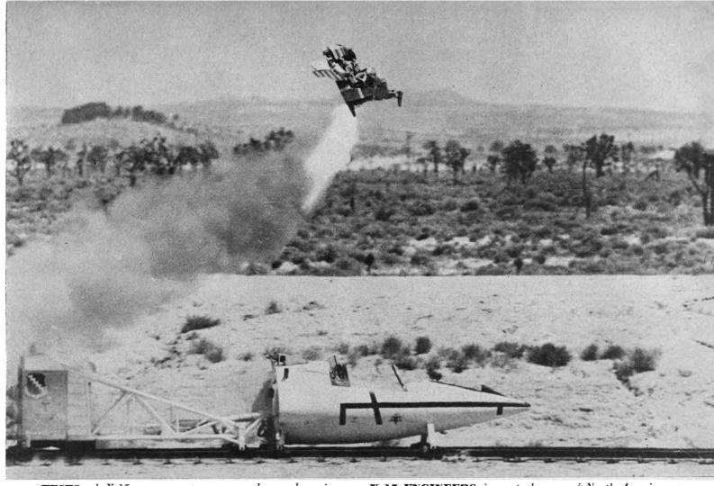
**TESTS** of X-15 escape system are made on dummies. Though pilot could not escape in space because he would burn, ejection is possible on re-entry into the atmosphere.
